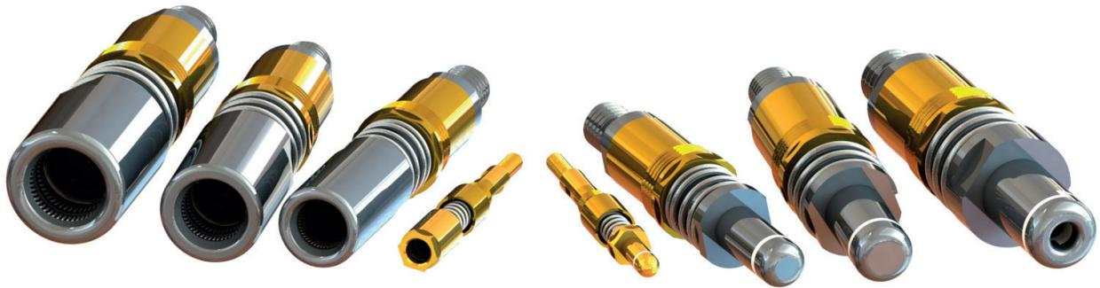
Round pins or round sockets are built into all new charging plugs for electric mobility all over the world. Therefore we offer solutions for common diameters (Ø4.0 / Ø6.0 / Ø8.0 / Ø10.0 mm). Other sizes are available on request.
