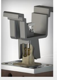
Not OK contact pins = abrasion/dirt
