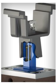
Not OK contact pin is bent No contact possible
