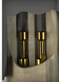
Abrasion/dirt = Spring contact pins' service life massively reduced
